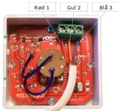
**Step 1:** Insert the white control cable into the left square socket.
