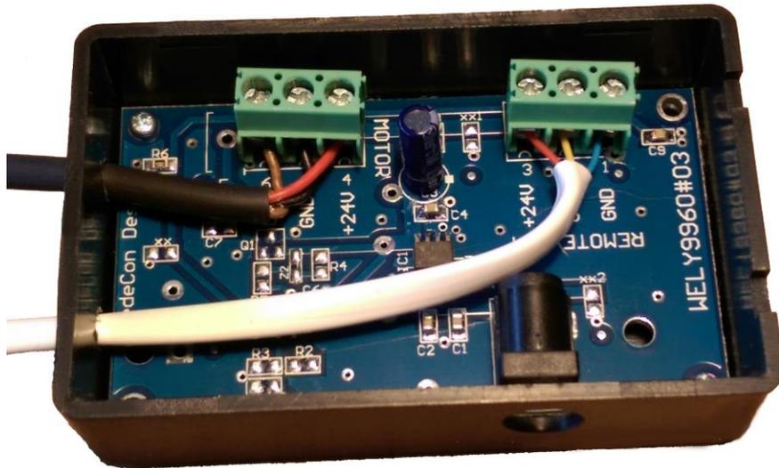
Mounting of control cable to control box:
