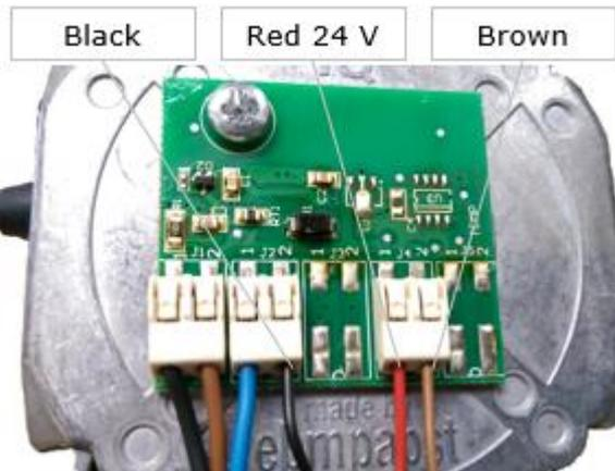
The cords are fastened to the terminals by pressing the terminal holders and at the same time pushing the ends of the cords into the terminals. See illustration.
